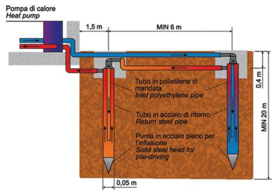
Recently, **Hydra** has produced a special application which can be fitted to its machines for the realisation of new concept geothermal probes for the heating/cooling of buildings.
